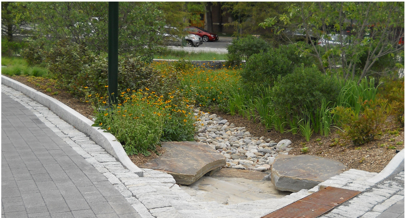
Green infrastructure best management practices (BMPs)—like this rain garden in Philadelphia, PA—utilize nature-based design to mitigate stormwater inundation and provide co-benefits such as improved water and air quality, wildlife habitation, and neighborhood beautification. BMPs contribute to sustainability and resiliency.
