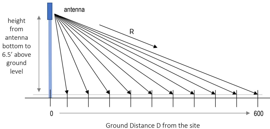
**Figure 2. Ground-Level MPE% Calculation Geometry**
